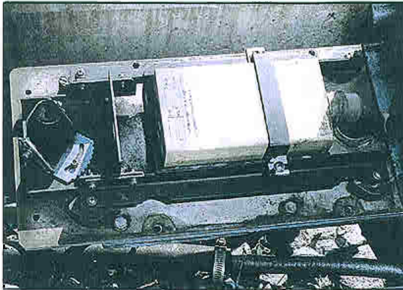
Figure 6-19: Scanner plate with pre-amp and reflector mirror
