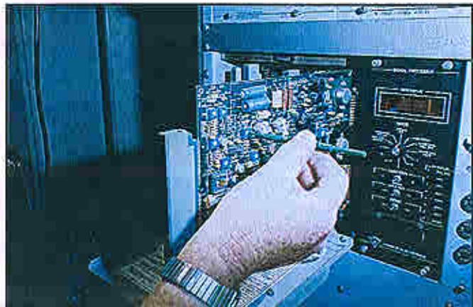
Figure 8-10: Adjusting the gain on rail 1 and rail 2
