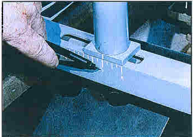
Figure 8-15: Looking through the peep hole to check the alignment
