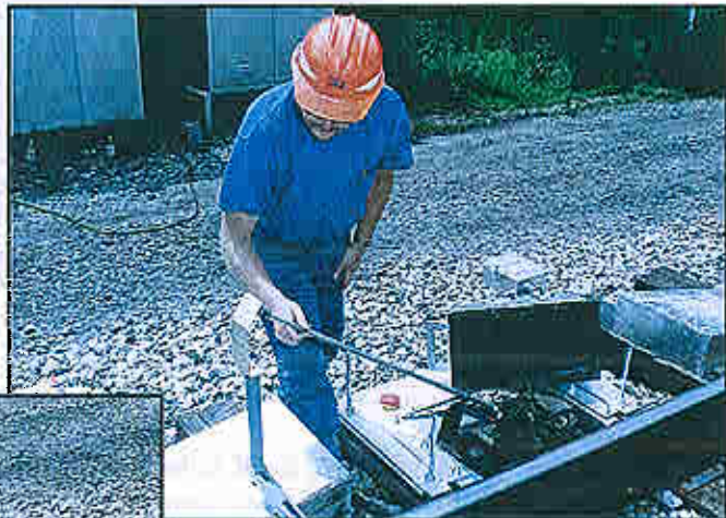
Figure 7-15: Measuring between the alignment fixture and the bolometer
