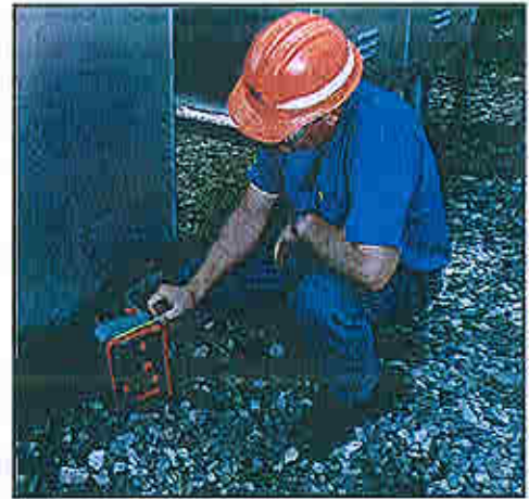
Figure 7-9: Placing the function simulator/generator and thermometer in shade
