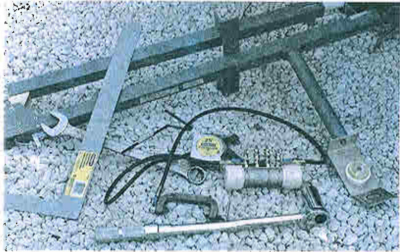
Figure 12-11 Tapeline, Alignment fixture, Mirror cap, Hardwire shunt, Appropriate hand tools.
