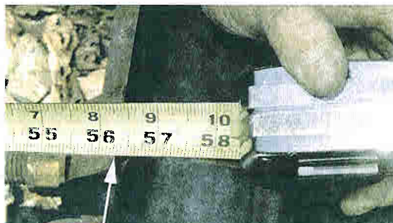
Figure 12-17 Verifying that the track gauge is still 56 ¼ inches.
