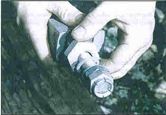
Figure 11-23: Scanner adjustment (cant nut)
