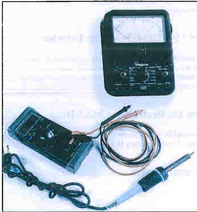
Figure 11-1: Fluke meter, Simpson 260, and soldering iron
