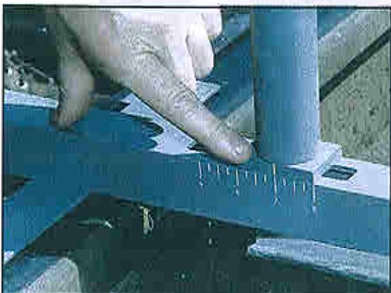
Figure 11-16: Adjusting to 7 inches \pm 1/4 inch
